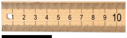
The numbered graduations are centimeters. There are 100 centimeters total in the meter stick. The unnumbered tiny graduations on the meter stick are millimeters. There are 1000 millimeters in the meter stick. As an example of using these units, the black line above is 44 mm, 4.4 cm, and 0.044 m.
